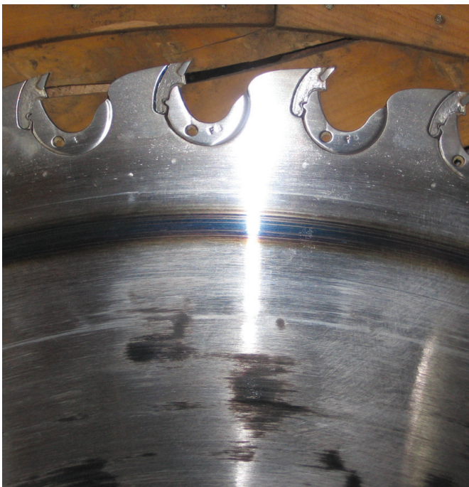
The blue streak tells a tale of overheating.
