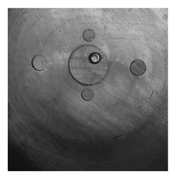
Standard 2" bore with two 5/8" pin holes on a 3" bolt circle and two 3/4" pin holes on a 5" bolt circle.
