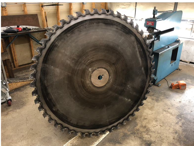
Notice the shiny guideline. This saw must have been running in and instead of fixing the problem, the sawyer chose to try and steer the saw with the guides.
