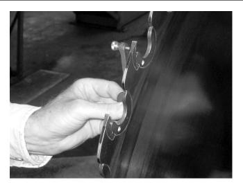
to adjust it to read the shoulder and also the part of the bit that is closest to the shoulder. This part of the bit is just the top of the bit body with no side grinding or kerf. If the bit body checks out okay and the shoulder checks out okay, meaning the same from side to side, then your problem is either number 1 or 2.
