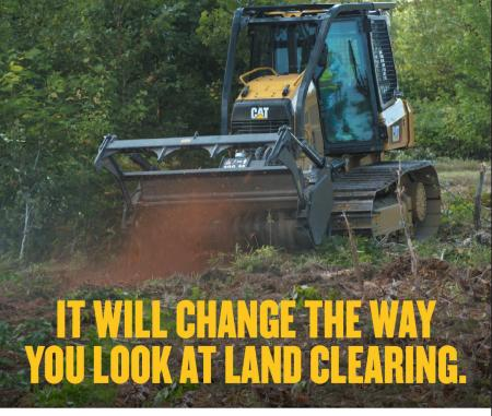
The CAT D3K2 Mulcher is an integrated machine/work tool package with a seven foot drum and both angle and tilt functionality on the mulching head. The high horsepower CAT engine gives you the power you need to handle just about anything you come across.
