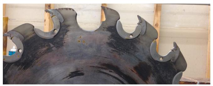
If just one socket is causing the problem, have a saw doctor replace it. More than one? Get a new edger saw.
