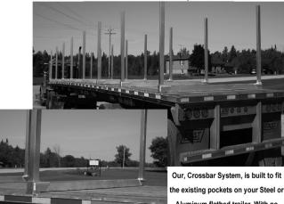
Unique center web design makes the Alum-A- Log Stakes 50% stronger and 50% lighter than most steel stakes. One Crossbar and 2 stakes only weigh 91 lbs. Aluminum flatbed trailer. With no alterations to your trailer.
