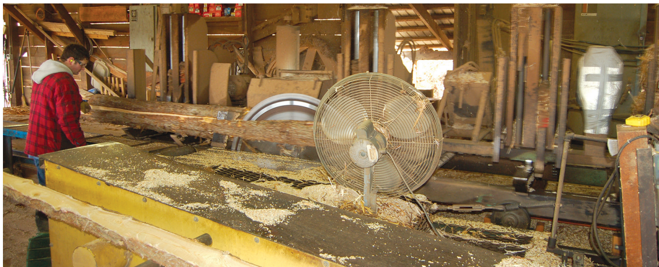
Saws need to run at the right speed for the material they're cutting—in this case, white cedar.
