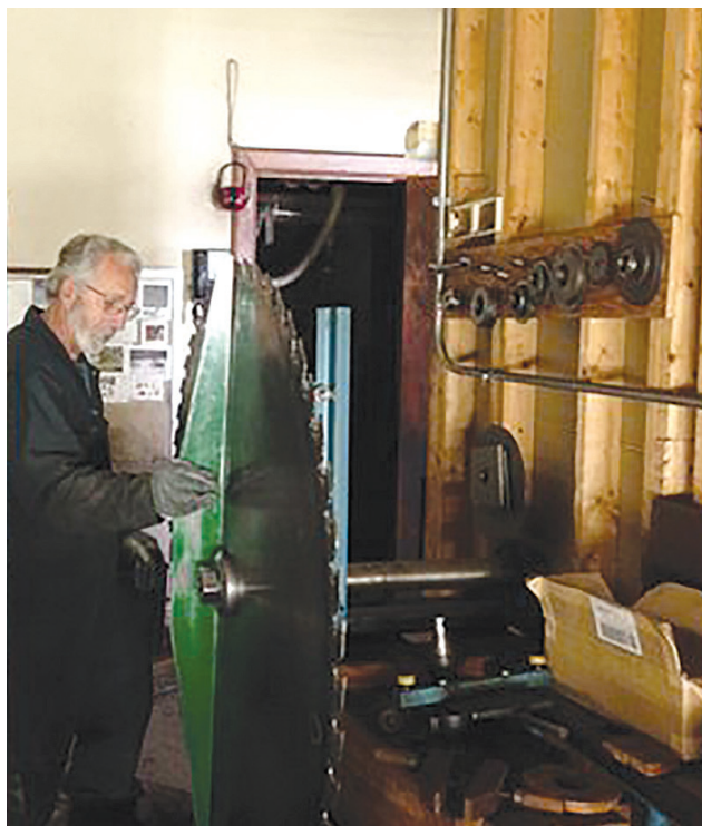
A sawmaker's straightedge is a precision tool.
