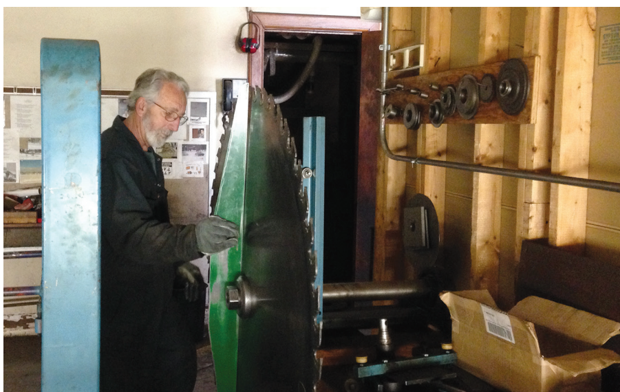
Creamer checks the vertical position to make sure it is flat on the log side and NOT dished in either direction.
