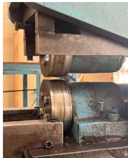
Left to right: The original convex rolls that came with my 3-60-C Stretcher Roll; my special retrofit rolls: leveling position and tensioning position
