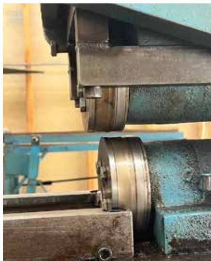
Left to right: The original convex rolls that came with my 3-60-C Stretcher Roll; my special retrofit rolls: leveling position and tensioning position
