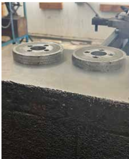
Left to right: The original convex rolls that came with my 3-60-C Stretcher Roll; my special retrofit rolls: leveling position and tensioning position
