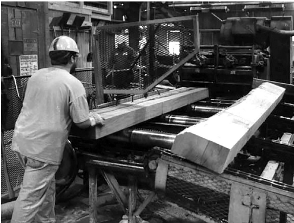
Cants and flitches need to be sawn square if they're going to be processed on a linebar resaw (below).
